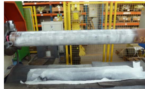
Bild 14: Rohr (Fa. VAM Drilling Inc.) gemäß Zeichnung B+V, Landing String 6.5/8" with 6.906 inch Slip Proof Section, Belastung 0 shtons - > 1250 shtons, Spannungserlauf \sigma = \sigma(t) [N/mm²], RxA_A = Messstelle, SS1 = Hauptmessspannung 1 Fig. 14: Drill pipe (PAM Drilling Inc.) acc. drawing B+V, Landing String 6.5/8" with 6.906 inch Slip Proof Section, load 0 shtons - > 1250 shtons, tension \sigma = \sigma(t) [N/mm²], RxA_A = gauge, SS1 = mainmeasurion 1
