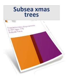
IOGP S-561 is based on API Spec 17D subsea wellheads and XT requirements.
