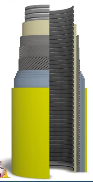
**Carcass** – Inner metallic layer prevents collapse due to hydrostatic pressure
