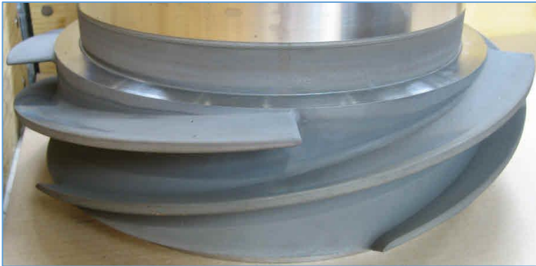
Coating on pump hydraulic stages
