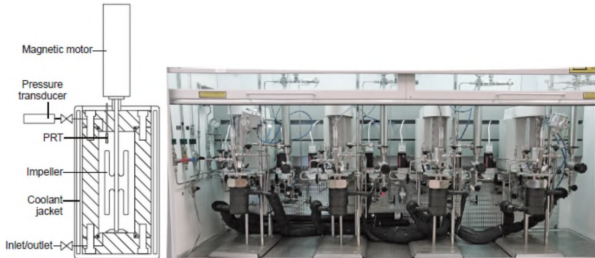
Figure 5 – (Left): Schematic representation of one “hydrates cell” used to study hydrates up to 200 bara and which can work at either isochoric or isobaric conditions. (Right): photograph of the 4 cells set
