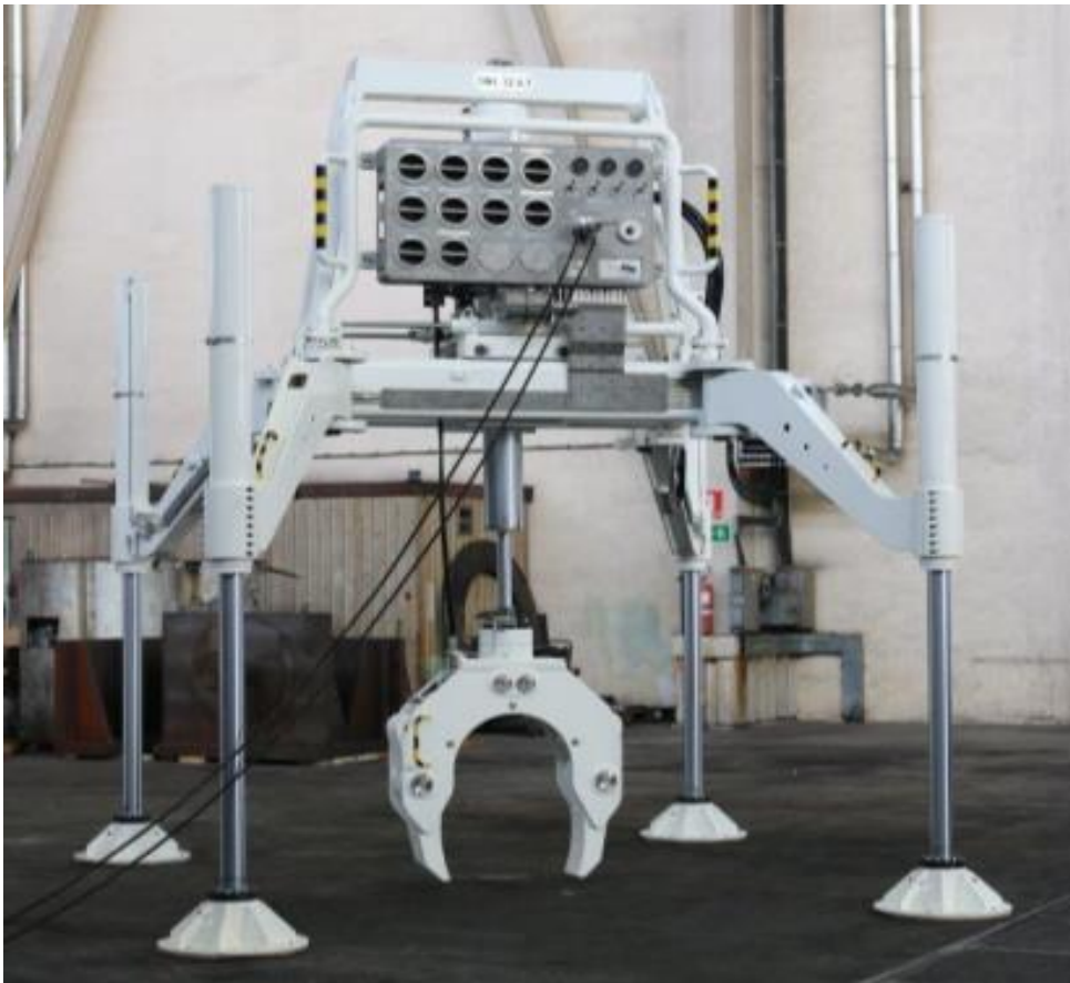
Figure 3: Remote pipe lifting frames supplied as part of the Petrobras CRD pipelines repair system. Rated up to 2000m, have been used in over 700 free span correction operations
