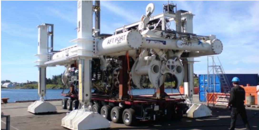
Figure 6: Statoil Coupling Installation Frame (CIF) with integrated pipe handling suitable for 6" - 30" pipelines
